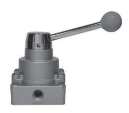
SHV-Series sliding hand valves are 4-way, 3-position, rotary disc, manual-operated air valves. Recommended for stationary air cylinders, arbor presses, and/or as a throttling valve for positioning air cylinder.
