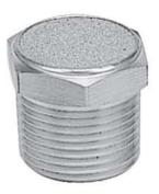
BV-Series low profile breather vents have many applications. They are most often used on single acting cylinders or valves to prevent dirt and foreign particles from entering ports open to the atmosphere. Common uses can also be found on vacuum relief or pressure equalization for gear boxes, crank cases, storage tanks or other vessels whenever pressure equalization is required.
