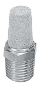
BM-Series mufflers utilize porous sintered bronze filter element secured to BRASS pipe fittings. These compact and inexpensive mufflers are furnished with standard male pipe thread connections, they are easy to install and maintain, particularly suitable where space is limited. They are used to diffuse air and muffle noise from the exhaust ports of air valves, air cylinders and air tools to an acceptable level within OSHA noise requirements.
